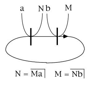
The new circuit has inputs **a** and **b**, and outputs that can measure the values of **M** and **N** without affecting the balance of the circuit itself. By choosing **a** marked and **b** unmarked, the memory is forced into the state (M,N) = (marked, unmarked). By choosing a unmarked and b marked the memory is forced into the state (M,N) = (unmarked, marked). In each case, since these states are stable, the marked input can be removed without affecting the state of the memory.
