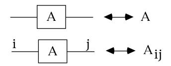
Matrix multiplication is represented by attaching the output line from one box to the input line of the other box.
