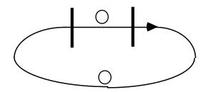
Each mark in the memory is unbalanced. The first mark to transmit a marked state will win the race and propel the memory into one of its two stable states. If it is possible for both marks to "fire" at once, we would arrive at the other unstable state where both sides are marked. In physical practice this will never happen, and the above unstable state will fall to one or the other of the two stable states, just as it does in our transition model (where one mark reacts faster than the other).
