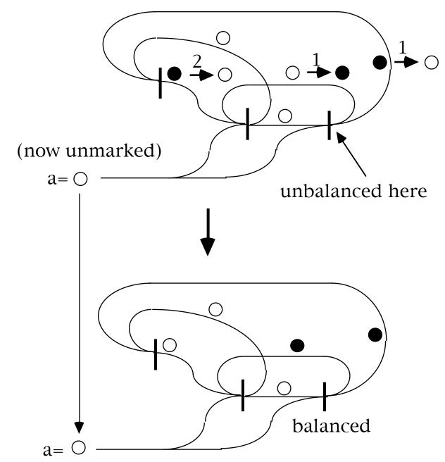
In the diagram above, we show how the change of a to the unmarked state gives rise to a transition of M to the marked state (1) and that this forces a transition of I to the unmarked state (2). The resulting circuit is balanced and the transition to this state of the memory is determinate.
