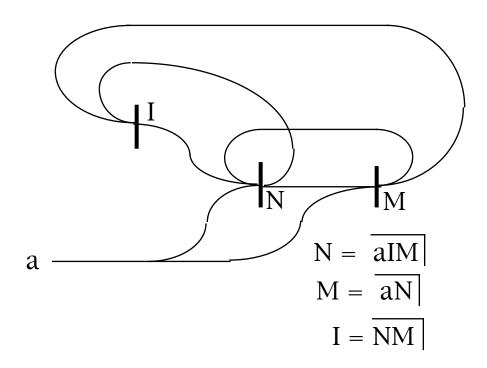
In this circuit we have eliminated the arrows that indicate direction of signals through the inverters and have used the convention that *signals travel through each inverter from left to right*. This suffices to fix all other directed lines. The memory consisting of M and N has an input a, and there is one more mark in the circuit labeled I. If a is marked, then N and M are unmarked, forcing I to be marked. This is a stable condition of the circuit so long as **a** is held in the marked state.
