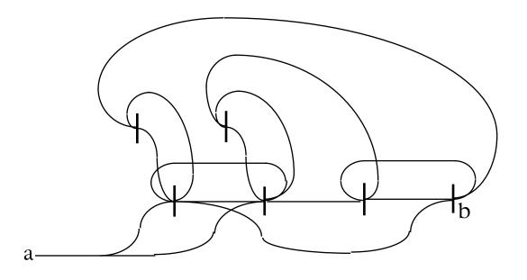
To see how this circuit operates, I have illustrated one stable state and one transition below. In showing the transition, I have only shown the end result. The reader will find that this is an example of a determinate transition. Note also that in the next transition, the value of b will not change. There is a four-fold cyclic pattern in the transitions, with b changing every other time.
