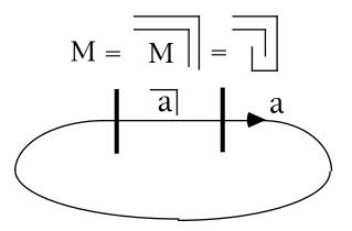
Here we have a benign reentry that does not create oscillation. The circuit has two stable states, and it is described by two equations with the extra variable N corresponding to the internal line in the circuit.
