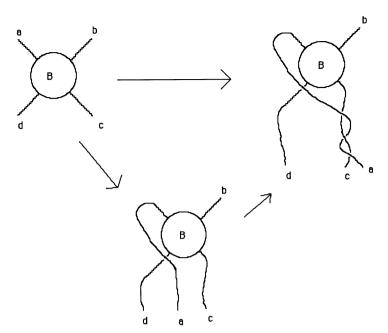
FIG. 2.2. Twining diagonally opposite strands via twists of adjacent strands.
