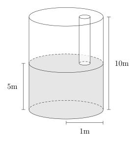
(a) Set up and evaluate an integral representing the work needed to pump the water out of the tank through the hose. The density of water is  $1000 \text{ kg/m}^3$ , and you may assume that the acceleration due to gravity is  $10 \text{ m/s}^2$ .
